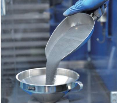
After series of complicated process as metallurgical, hydrogen reduction and carbonization, the tungsten carbide powder is our raw material of RTP powder. Over 30years rich experiences and technology developing on metallurgy, we owned comprehensive grades which almost cover all the machining applications, included the upgrade nano grain size made of tungsten carbide powder as fine as 0.2um.
