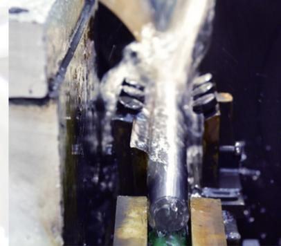
According to different applications and customer requirements, cemented carbide products need to go through finishing processes such as grinding to meet the required size and accuracy. We always control the grinding accuracy with more tight tolerance.
